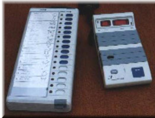
**Figure 1:** Electronic voting machine & control unit
